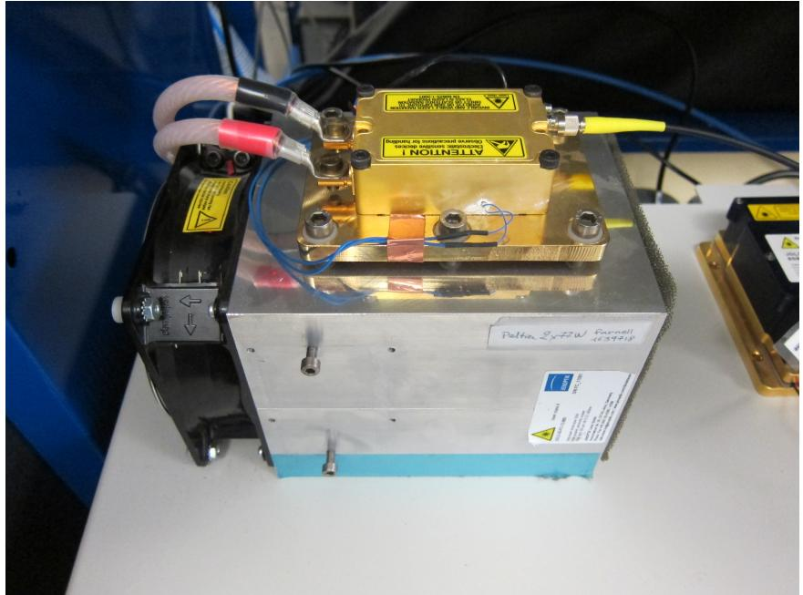
Laser diode (25 W- emission at 880 nm ) - connected to an optical fiber of 200  $\mu$ m.
